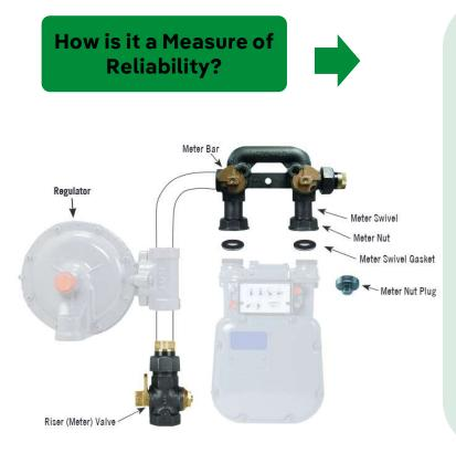
Recall, NYSEG and RG&E combined serve approximately 593,000 gas customers. Every customer has a connection to the gas distribution system known as a gas service. For pressures greater than Low-pressure, customers will have a gas regulator to reduce delivery pressure to 7-8" WC.
