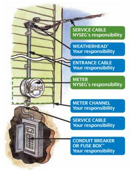
\* WEATHERHEAD (Service Head) - A type of conduit used to prevent entry of rain into the service entrance cable.
